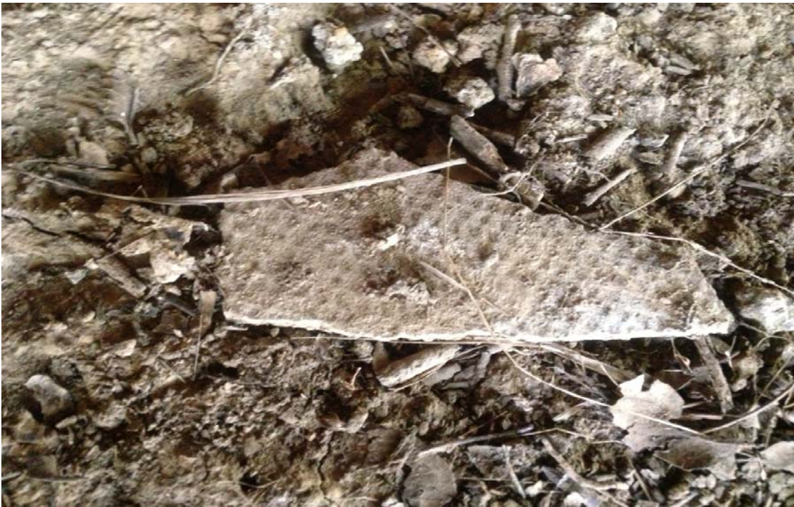
Photograph 6 – Example of Asbestos containing material fragment.
